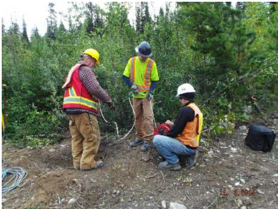
Photo 2: Amec Foster Wheeler Construction Monitor measuring depth of well.
