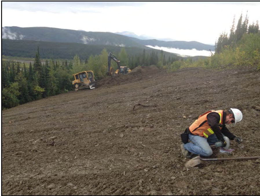
Photograph 35: Amec Foster Wheeler carrying out confirmatory XRF sampling on final surface of decommissioned Jewelbox switchback (August 29).
