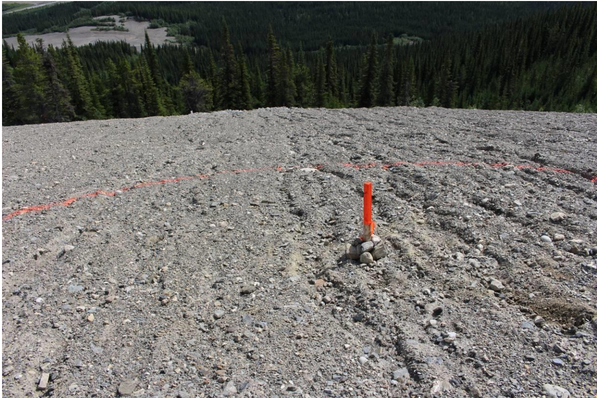
Photo #18: Plot GP-3 showing the steepness of the site and the rilling on the slope.
