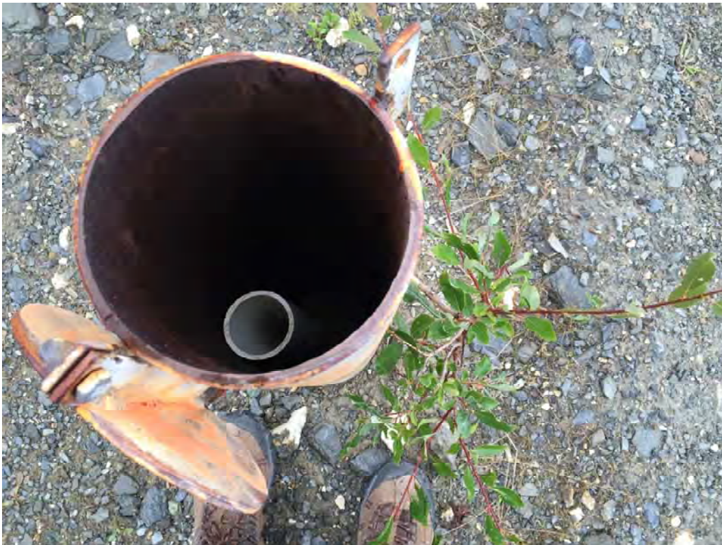
Photo 4 PVC Piezometer Inside the Protective Caps
