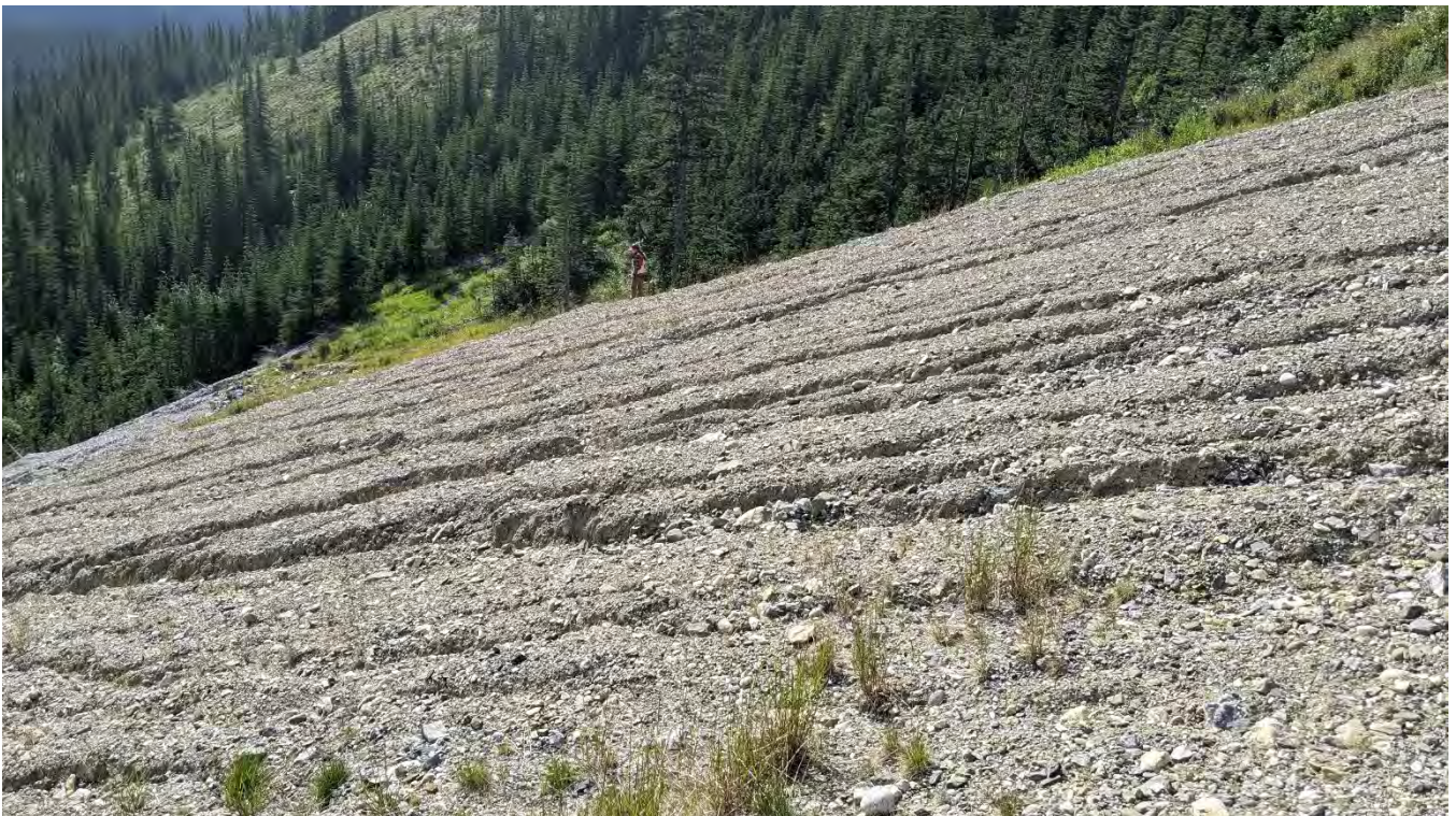
Photo WR-12: Rill erosion at the south end of the 1408 Portal Waste Rock Dump looking southeast.
