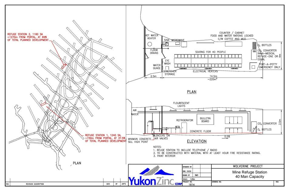
Figure 2-3: Underground Mine Refuge Station
