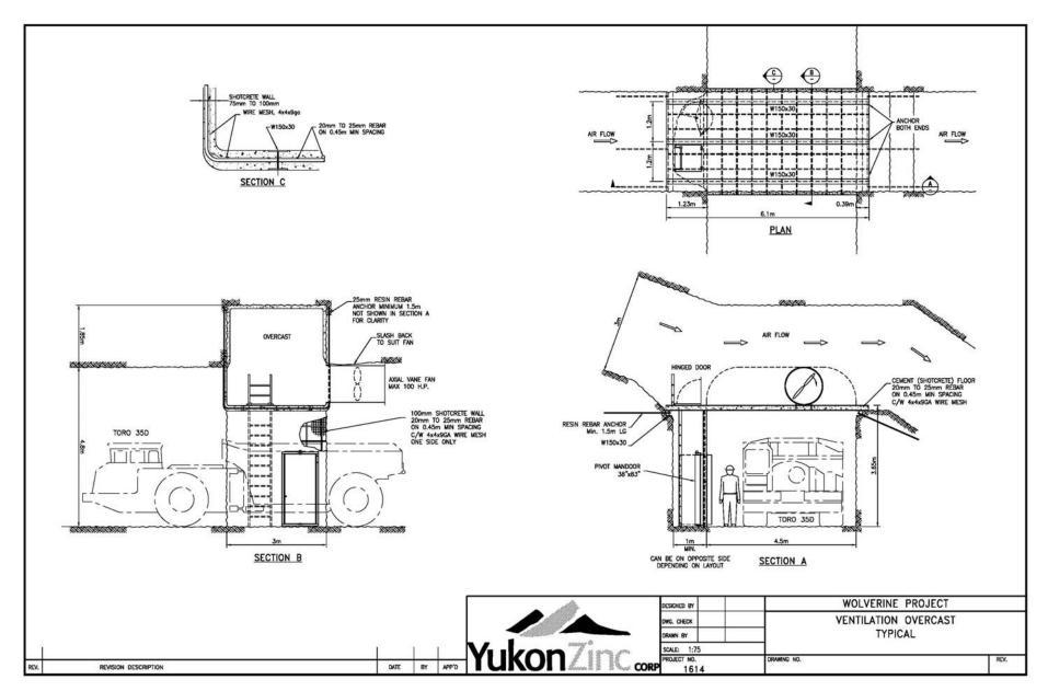
Figure 2-4: Plan View and Sections Through Typical Ventilation Overcasts
