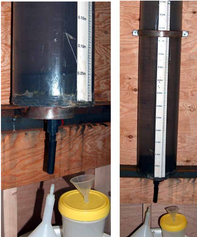
Figure 1.22 Set-up of Sub-aqueous Columns
