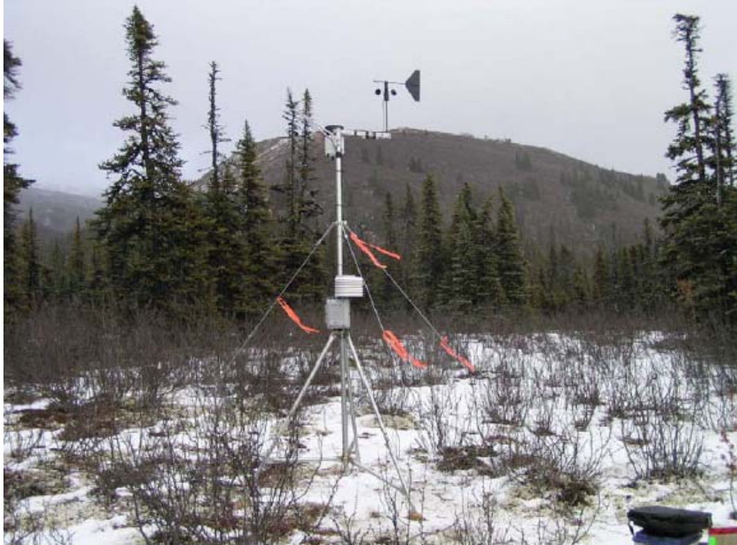
Figure 7.1-3 Automated Weather Station Located Near Airstrip
