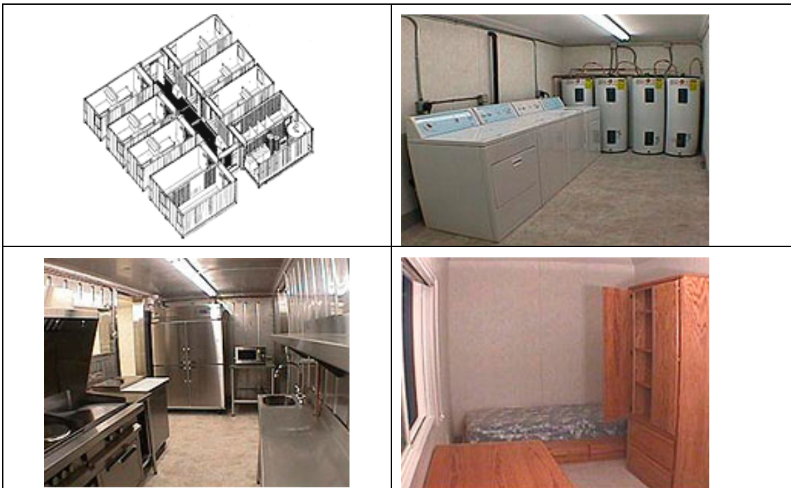
Picture 2.3. Example of the configuration and interior of a modular construction camp comprised of pre-fabricated sea can containers.
