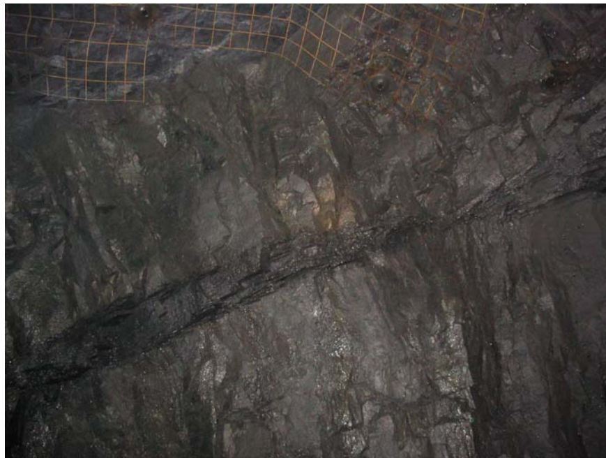
Photograph 22: Location 7 View of the wall - Note the contact between massive ore zone and an argillite band in between.
