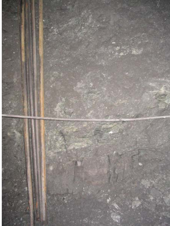
Photograph 21: Location 6 View of the right wall in the massive sulphide with internal argillite bands in the bottom part and argillite in the upper part.
