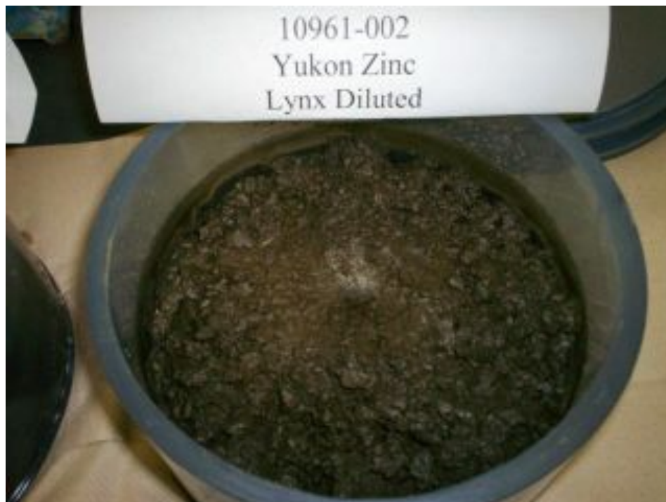
Photo 3: Lynx Diluted Tailings in the Humidity Cell (October 6, 2006)
