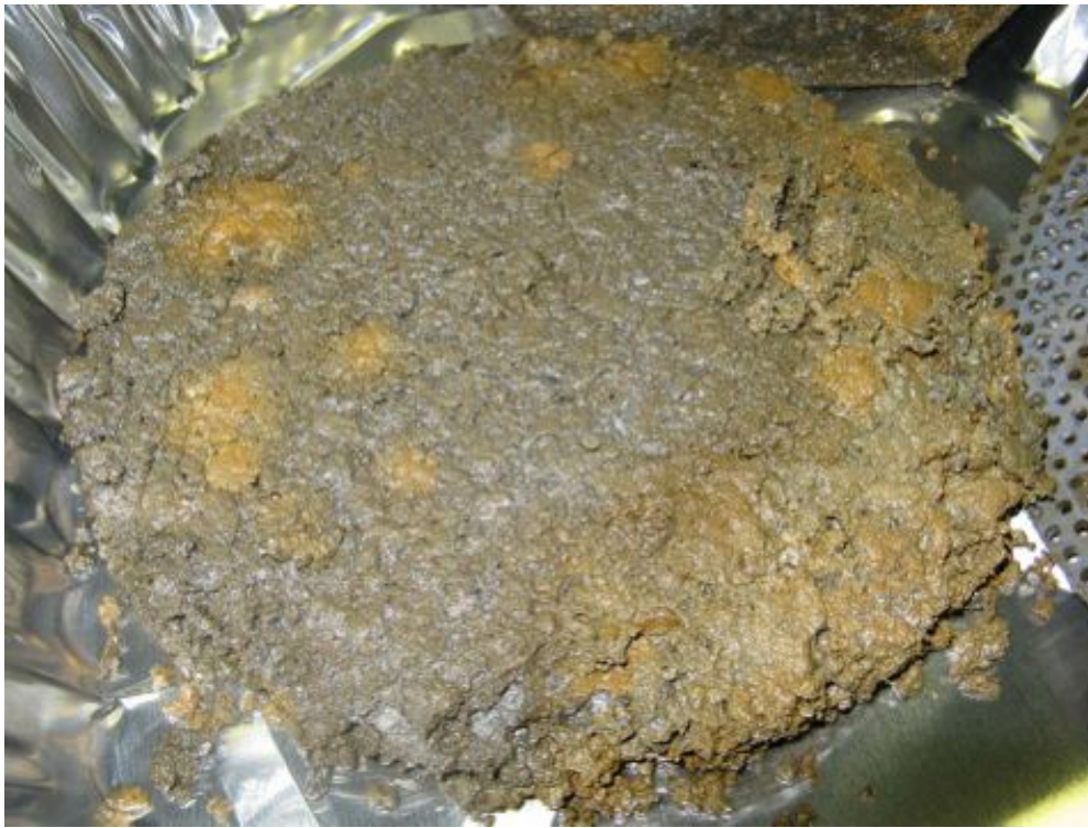
Photo 5: OD Tailings Sample Placed on Sheet for Drying (January 29, 2012)
