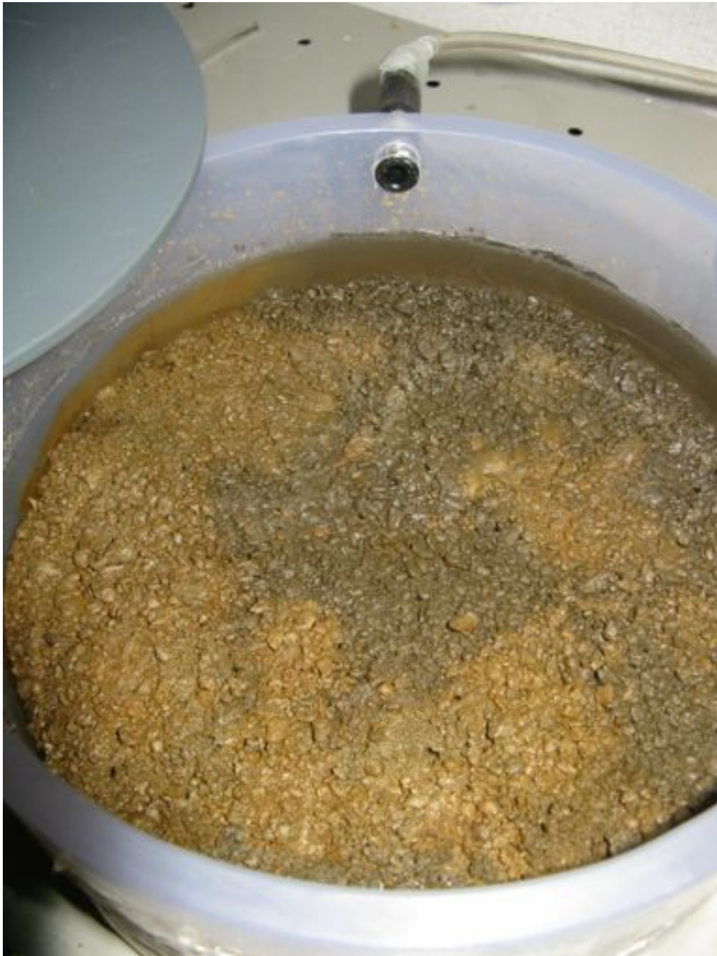
Photo 4: OD Tailings in the Humidity Cell (January 29, 2012)
