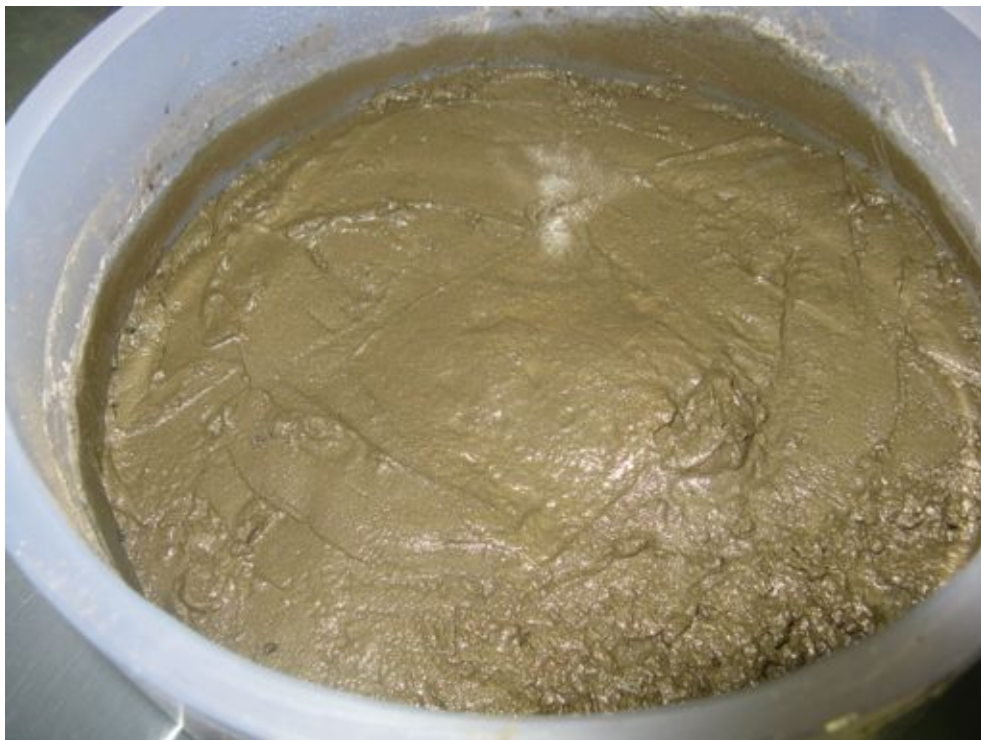
Photo 6: OC Tailings in the Humidity Cell (January 29, 2012)
