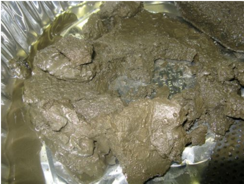
Photo 7: OC Tailings Sample Placed on Sheet for Drying (January 29, 2012)
