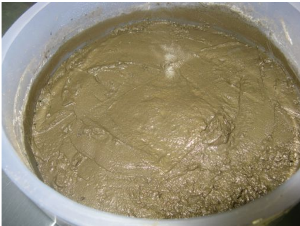
Photo 6: OC Tailings in the Humidity Cell (January 29, 2012)
