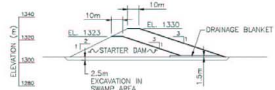
SECTION A TAILINGS DAM CROSS SECTION
