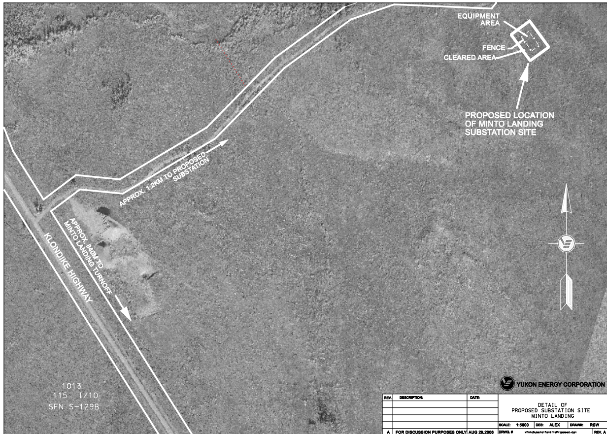
Figure 5.7-4 Footprint Conceptual Layout of the Minto Landing Substation
