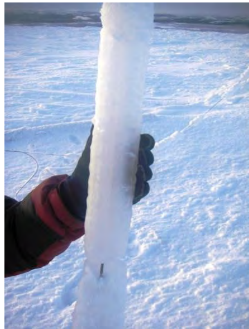
Figure 51 Rime Icing on Guy Wire of Collapsed Met Tower in Alaska
