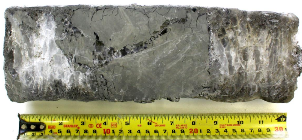
Figure 6.5 Ice-rich permafrost core taken from IV_BH1 at 6 m depth.
