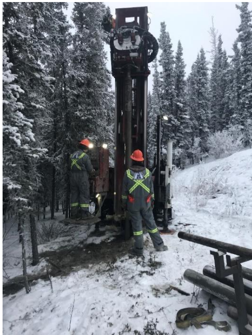
Figure 5.6 Midnight Sun Drilling at borehole HV_BH1 using a sonic drill.
