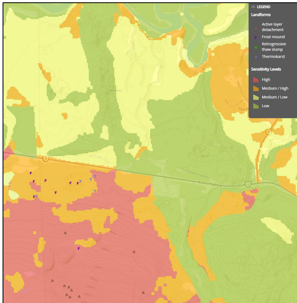
Figure 3. Sample of the permafrost thaw sensitivity webmap for the area near the junction of Alaska Highway and North Klondike Highway.
