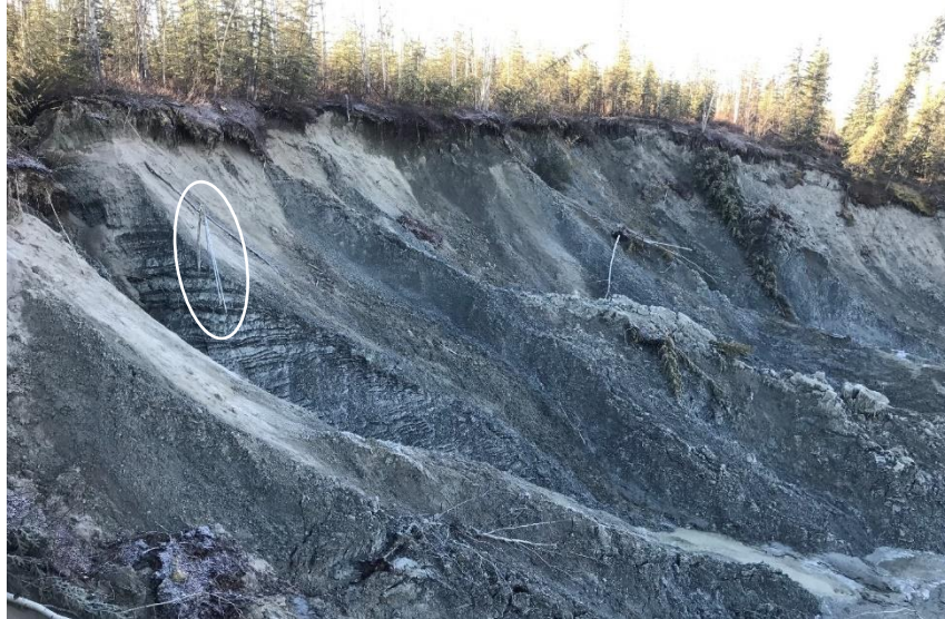
Figure 7.5 Roughly 8 m of laminated glaciolacustrine sediments are exposed in the thaw slump headwall near borehole WH_1456_BH3, 15 October 2020. Broken borehole casing is circled.
