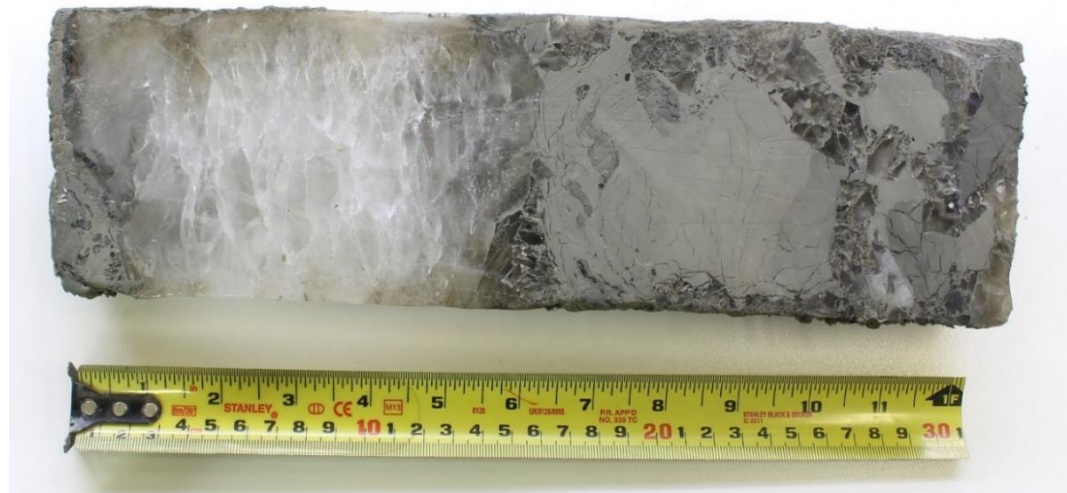
Figure 7.12 Ice-rich permafrost showing thick layered (left) and suspended (right) cryostructures in a core from WH_1456_BH1 at 6.57 m depth.
