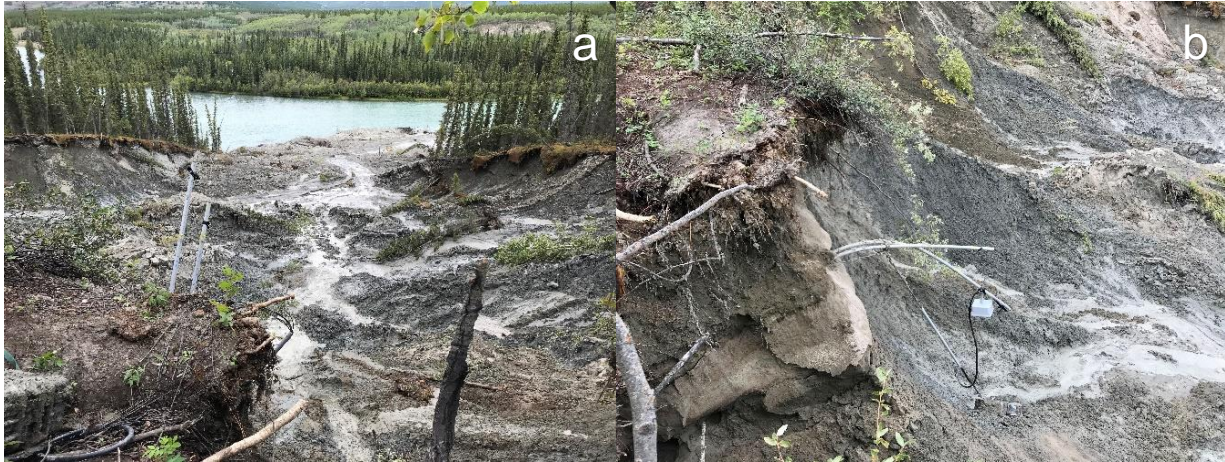
Figure 7.14 WH_1456_BH3 borehole casing and instrumentation (a) prior to, and (b) following collapse into the slump on 13 August 2020.
