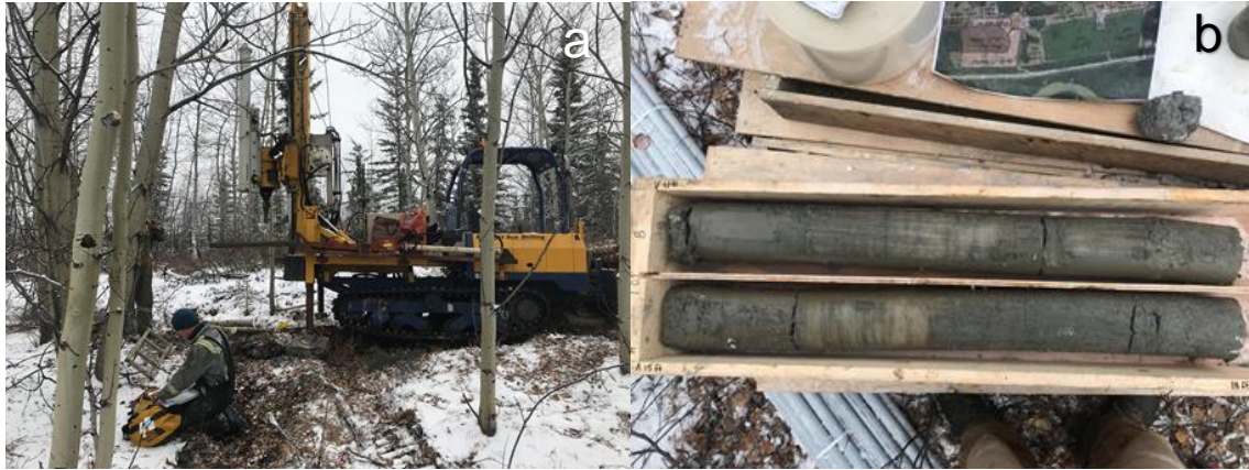
Figure 7.11 (a) Midnight Sun Drilling CRREL drill rig and (b) permafrost cores at WH_1456_BH1.
