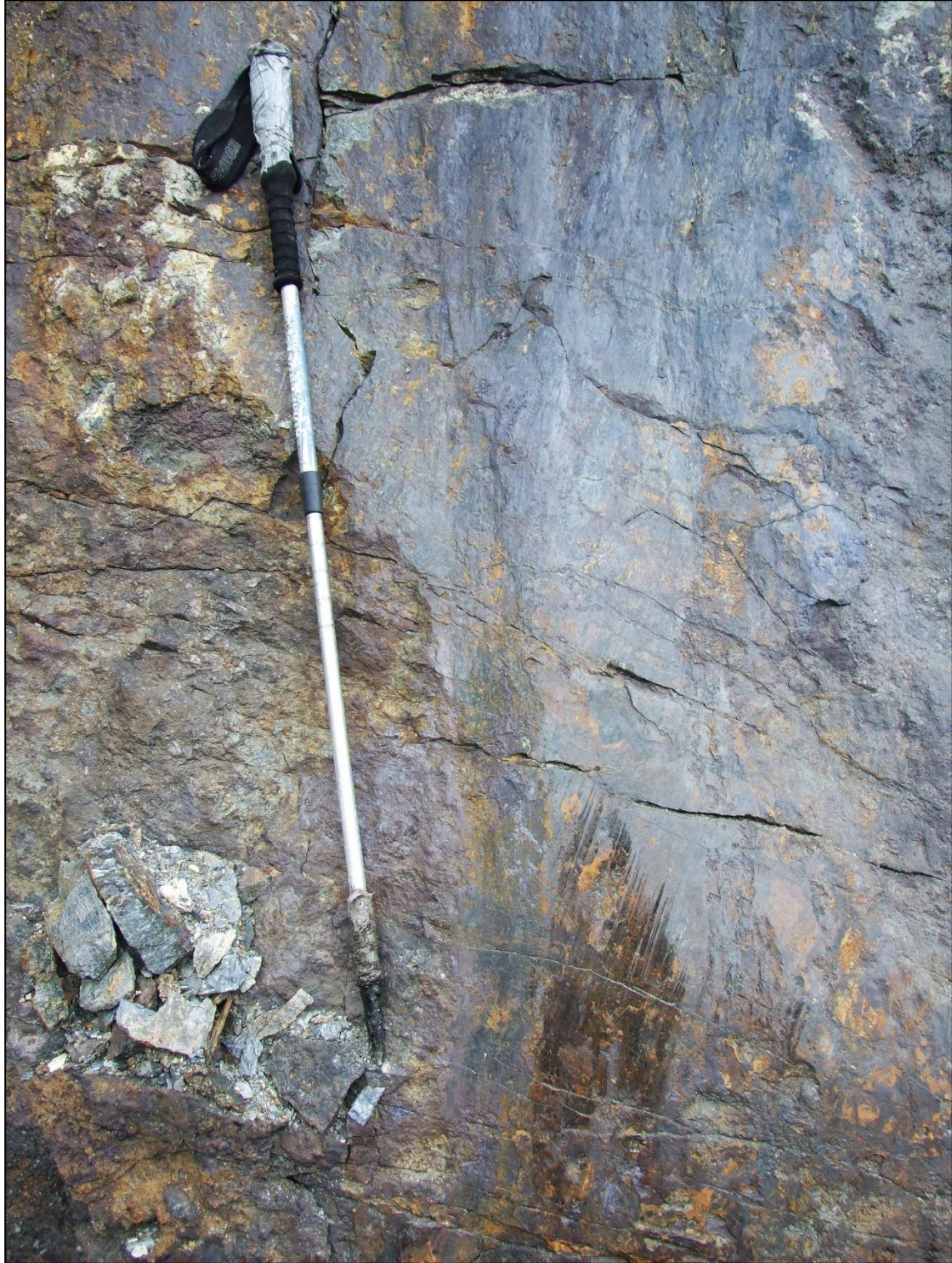
Photo 8. Fine post-mineralization slickensides on the No. 9 vein footwall.
