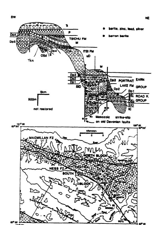
Stratigraphic section across the MacMillan Fold Belt (not restored). IC - Vampire Fm., ClO - Sekwi, Hess River and Rabbitkettle Fms., ODd - Duo Lakes Fm. Abrupt lateral changes in stratigraphy reflect syndepositional extentional and/or wrench faults. Mesosoic strikeslip of relatively small, but unknown magnitude along some faults complicates paleogeographic interpretations. The barite-sinc-lead deposits are spatially related to the faults.
