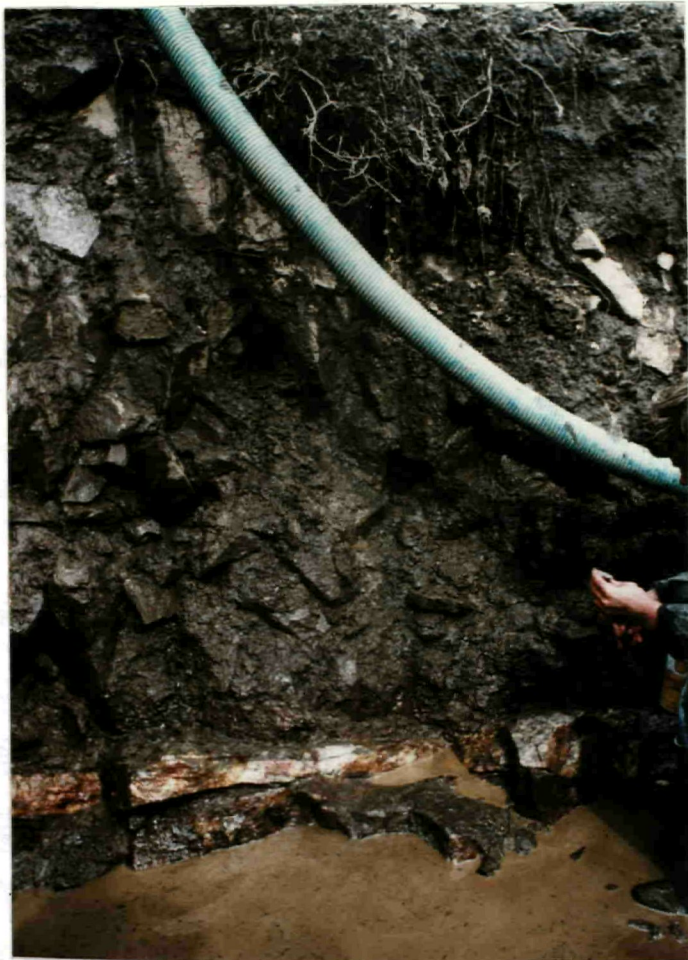
Typical vein intersection during trenching. Coarse blebs of gold are usually visible along weathered fractures after alteration of laminated sulphides.
