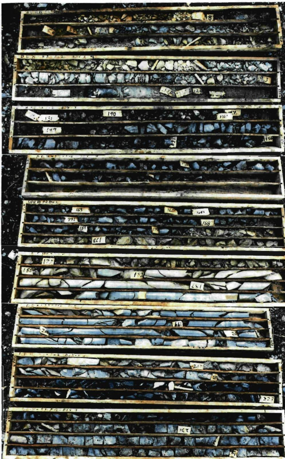
Photograph 6: Drill core from Hole 88-2; note poor recovery in top 47.6 m (156').
