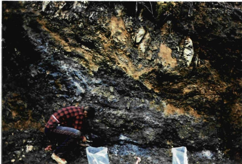
Photograph 5: Chip sampling of Trench P-11. Interval shown assayed 0.69 g/t Au over 1.7 m.
