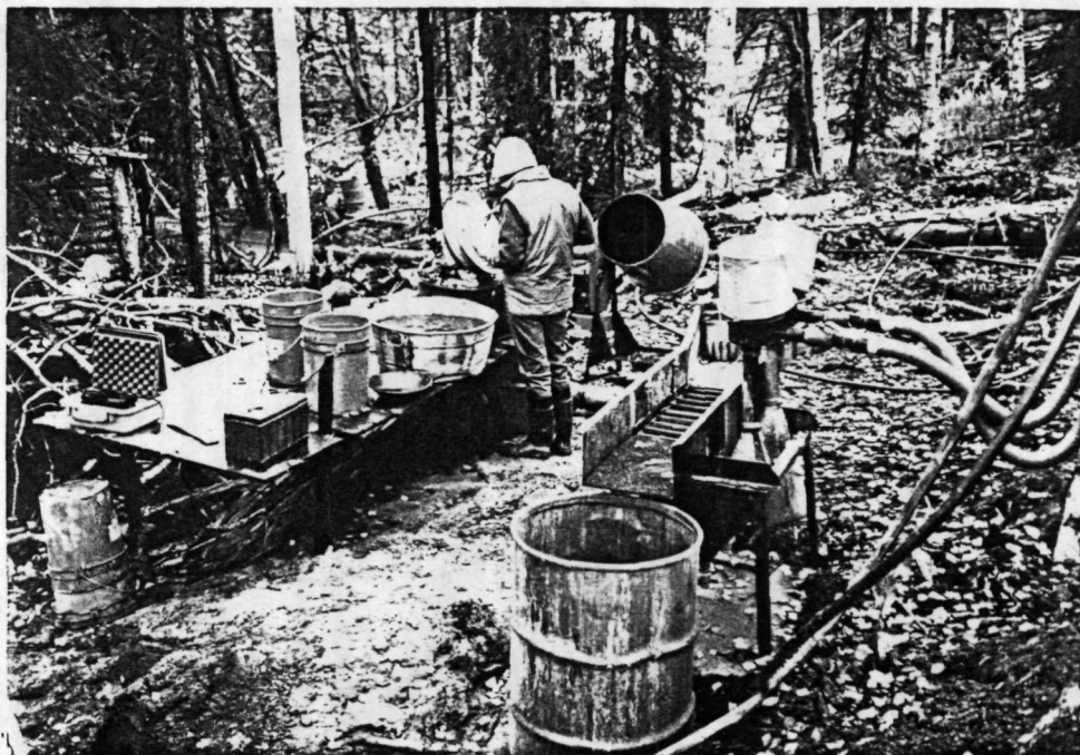
Concentrating area where individual bulk samples from hard-rock veins were processed. (Counterclockwise from right: Duplex PanAm jig; Amalgamating barrel; Mercury wheel; Retort; Panning tub.)
