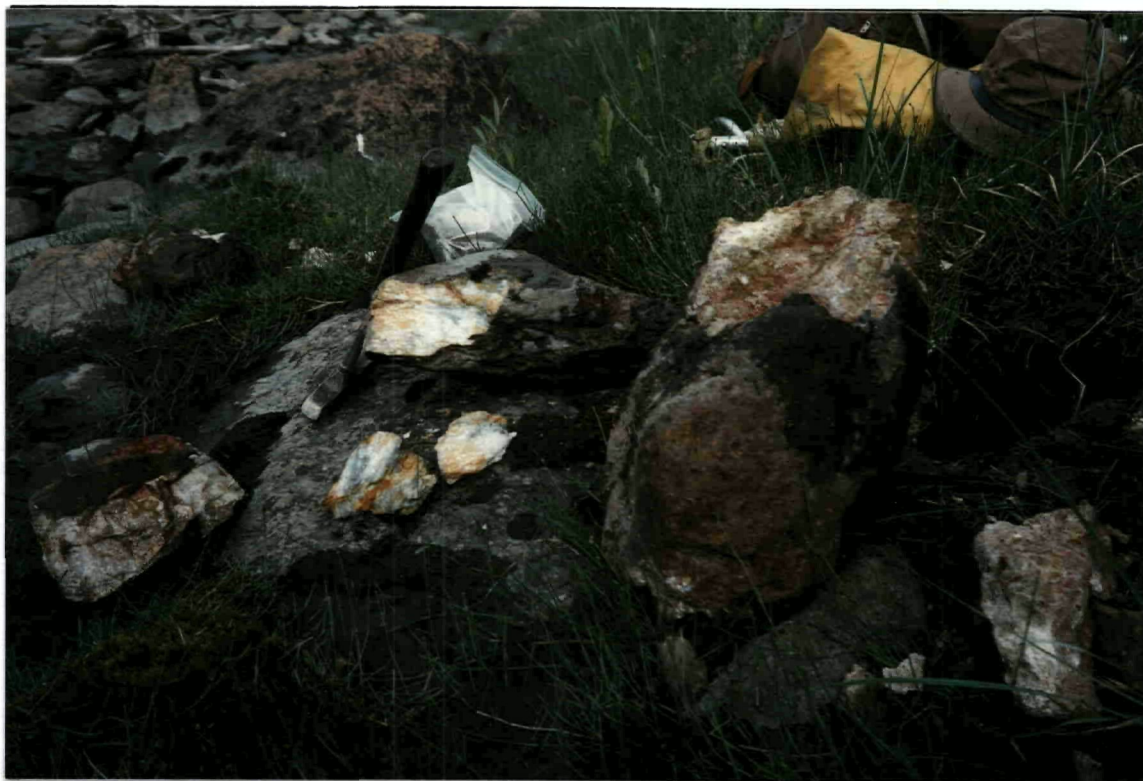
PHOTO 3 Sulfide-bearing boulders right bank of Hoole River 300 m up-stream from base camp. Center boulder NAL#14566 at 1.5% Cu. Quartz boulder left NAL#14562 332ppbAu, 2955ppmAs.
