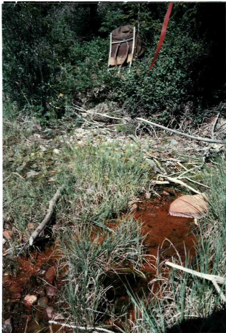
PHOTO 5 Typical limonite encrusted seepage issuing from evident fault zone parallel to right bank of Hoole River near UTM 575356. Several cobbles nearby display epithermal vuggy vein quartz with pyrite and minor arsenopyrite
