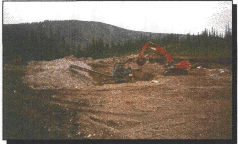
Floater Dredge working on frozen bench. Note the dredge pond behind the floating gravel processing plant.
