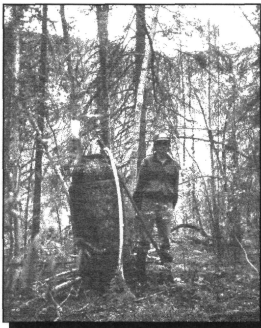
We found this old steam boiler complete with steam point and hose, used by hand miners to sink shafts.
