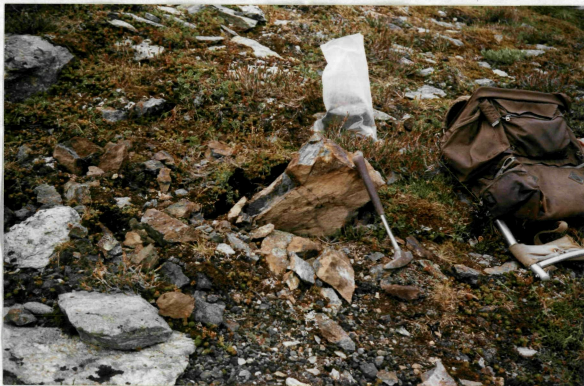
PHOTO 8 Sampling of subcrop pyritic muscovite-chlorite-schist at timberline south of basecamp valley at 1520 m 39870E/67986N
