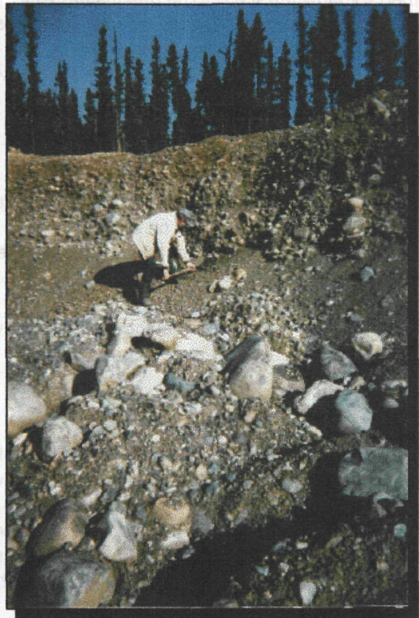
Collecting gravel samples in a borrow pit. The gravel in the foreground is typical of aggregate composition in the project area. Boulders are plentiful and the rock is rounded and well washed.
