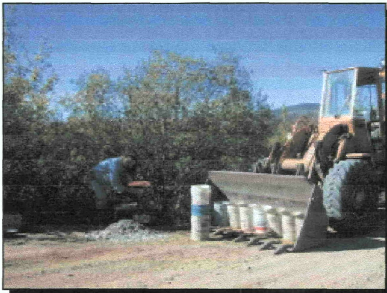
Processing gravel cuttings using a long tom sluice set-up. A rubber tired loader was used to transport samples, contained in 5 gallon buckets, to the processing site.
