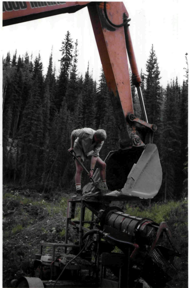
PROCESSING 1 yd 3 SAMPLE WITH SMALL TROMMEL / KNUDSEN BOWL.
