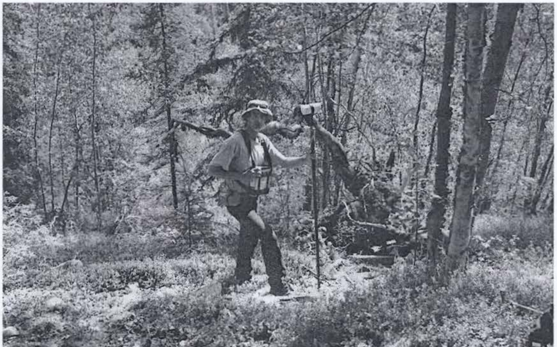
Photo 2: Ground magnetometer survey on the KIT 7 claim
