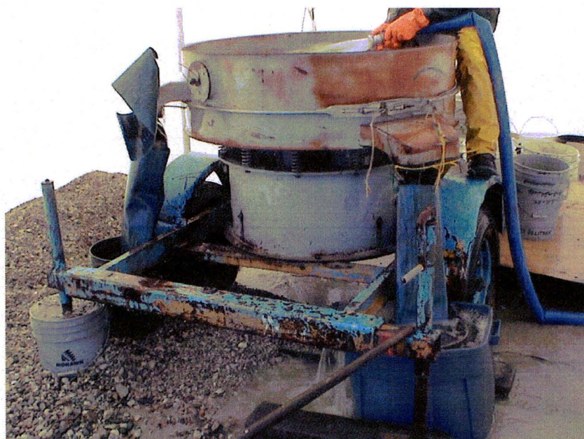
Photo 9: Samples being screened using a Sweco Separator.
