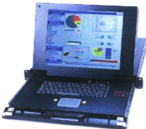
Figures 2 & 3: Geo-iMAGe Screen/Keyboard module comprising a 19", 1 "U" high, rack-mount drawer containing a folding 15" LCD TFT (1024 x 768 pixel resolution) screen, keyboard and touchpad "mouse" pointing device.
