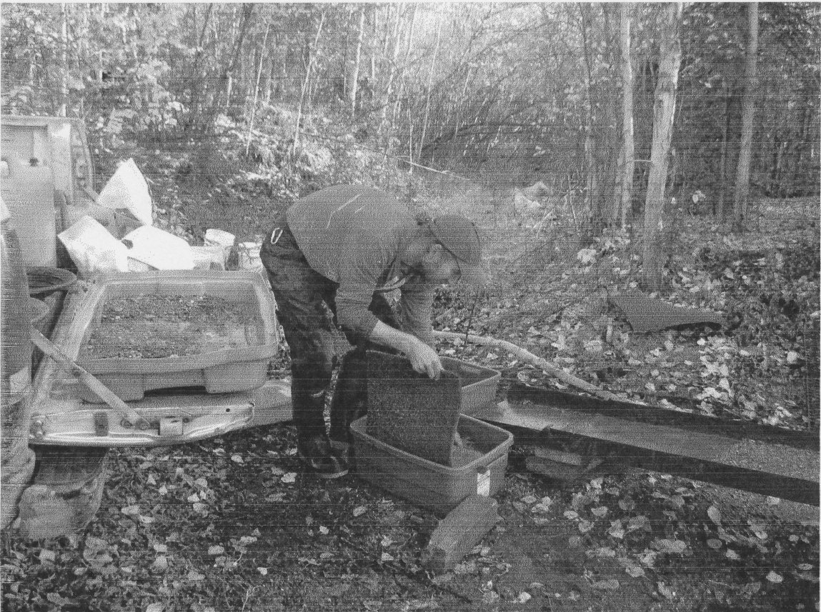
Long Tom Test Sluice at field camp
