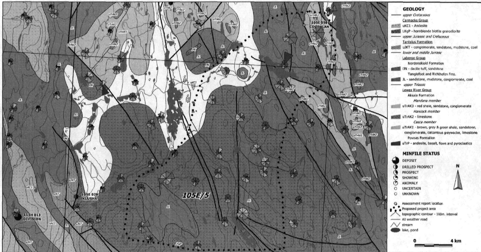
Figure 4. Geology (Gordey and Makepeace, 1999), Minfile number and name (Deklerk and Traynor, 2004) and Au, As, Sb, Hg, Ag, Cu, Pb, Zn RGS geochemistry (Heon, 2003) of the project area. Key to multi-element geochemical symbols is shown in figure 5. The Braeburn Fault is the fault roughly parallel to and west of the highway, Coughlan fault (Tempelman-Kluit, 1984) is the north northwest trending fault separating the Laberge and Lewes River Groups at the Coughlan Minfile occurrence. Belleview Mountain is approximately 4 km. east southeast of the Klusha Minfile occurrence. Braeburn Lake is the large north trending lake near the center of the map.
