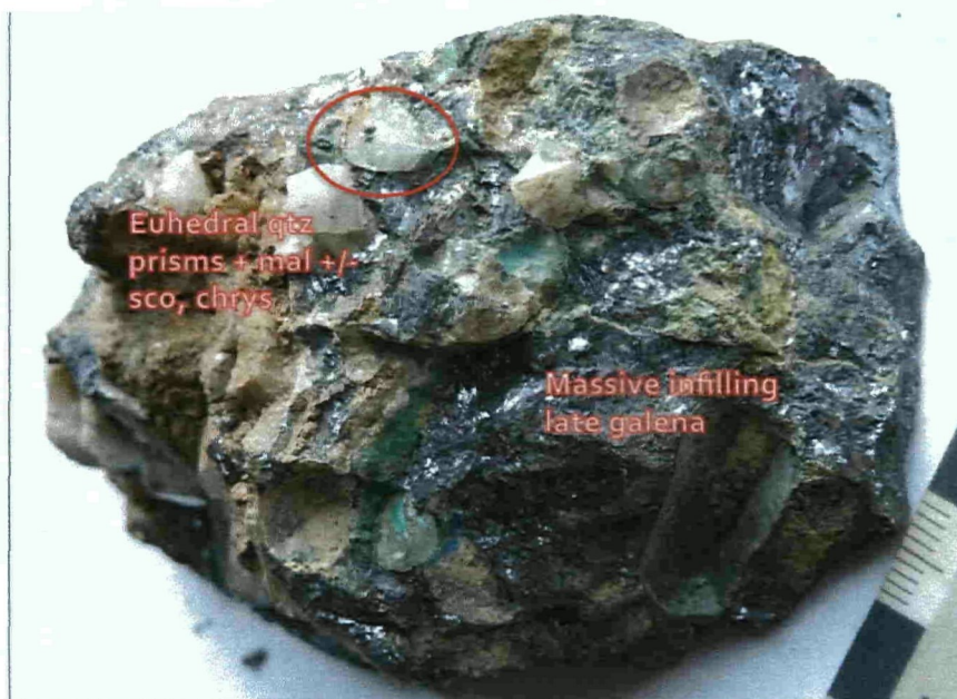
Figure 10. Euhedral quartz prisms with cubic galena inclusions surrounded in banded base metal mineralization (galena + malachite ± scorodite, chrysocolla).
