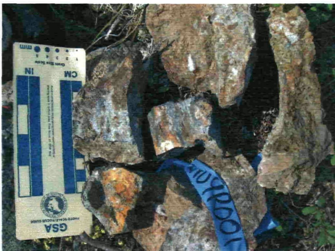
Figure 7. Rock sample RH09R001, brecciated schist – quartzite with quartz, iron oxide stain and boxwork texture.
