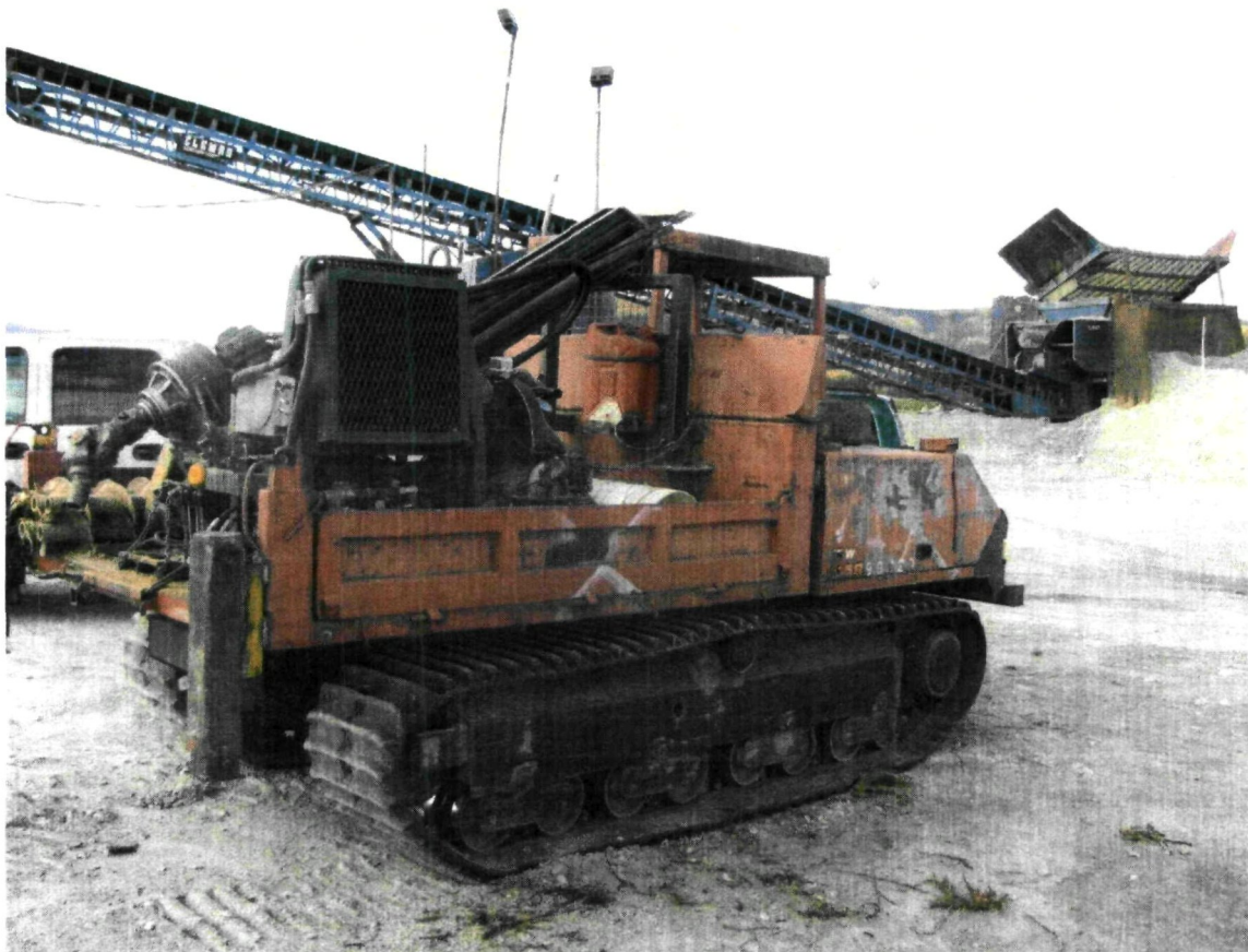
(Photographs 3 and 4. A. Hollis' gasoline powered hydraulic auger mounted on a rubber tracked Yanmar diesel carrier, photo taken by Tara Christie)
