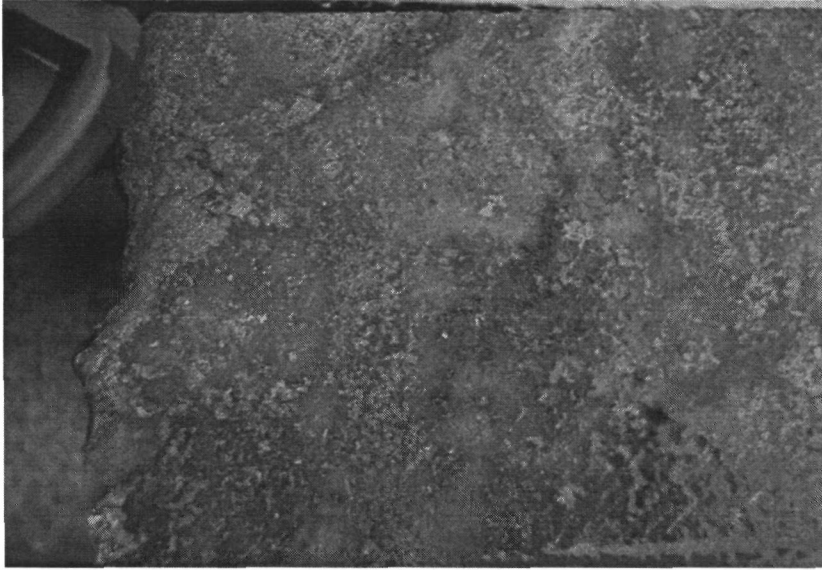
Figure 30. Pyrrhotite disseminated in skarn (in core)
