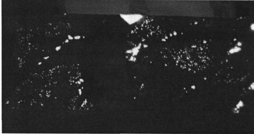
Figure 28. Grain size variation in scheelite mineralization (in NQ core)
