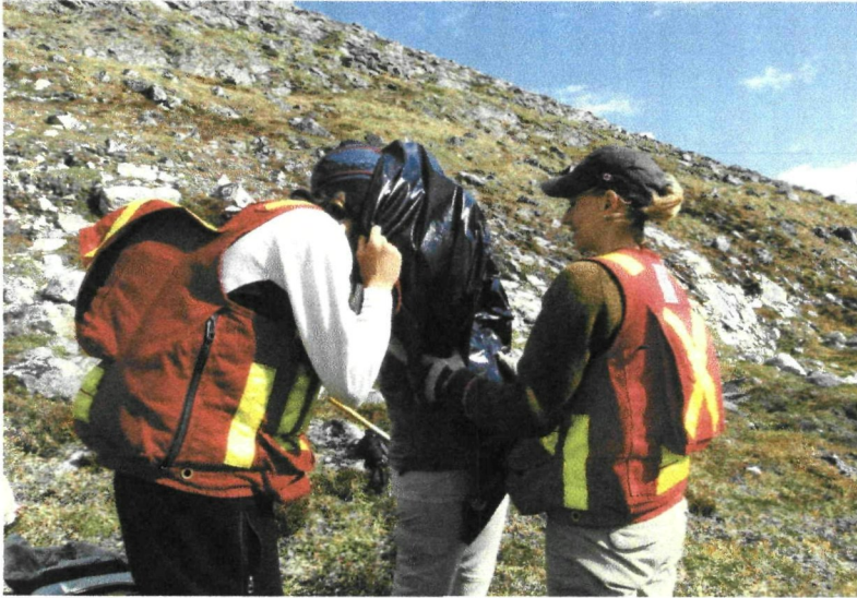
Field portable 'dark room' for assessing scheelite content
