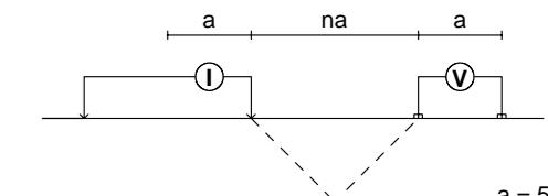
Stationary electrode at 10000E (moving W).
