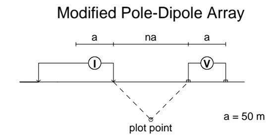
Stationary electrode at 10000E (moving W).
