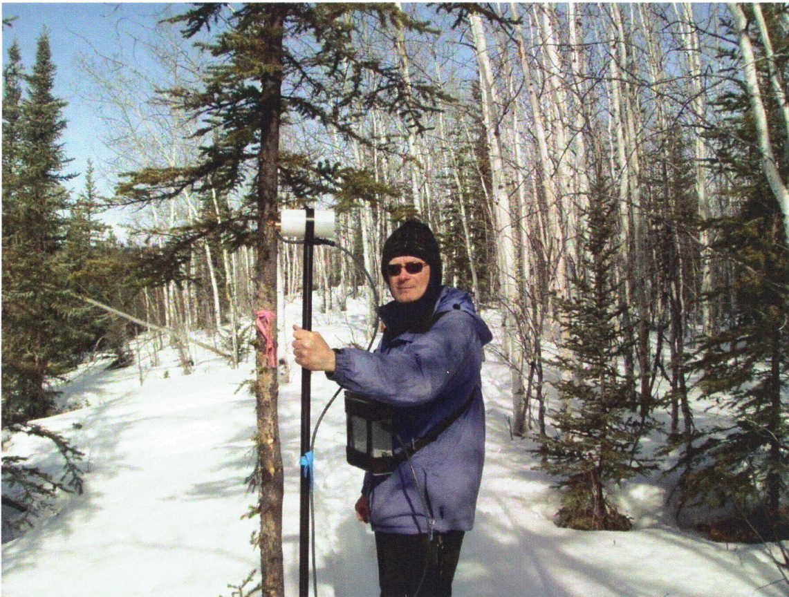
Magnetometer survey on the western edge of the glacial fluvial terrace. (Bob Stirling)
