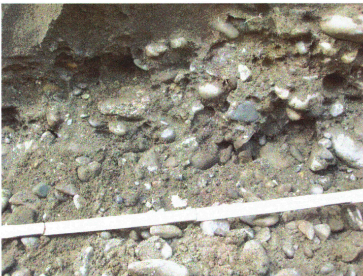
IC-TR-10-17: silty sand matrix, granitic bedrock erratic
