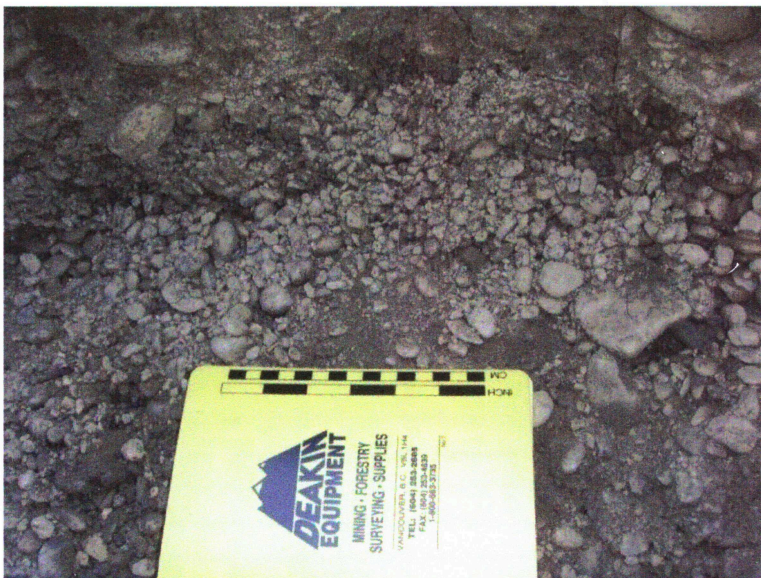
IC-TR-10-10: rounded stacked pebbles intermixed with larger gravel to 14 inches diameter
