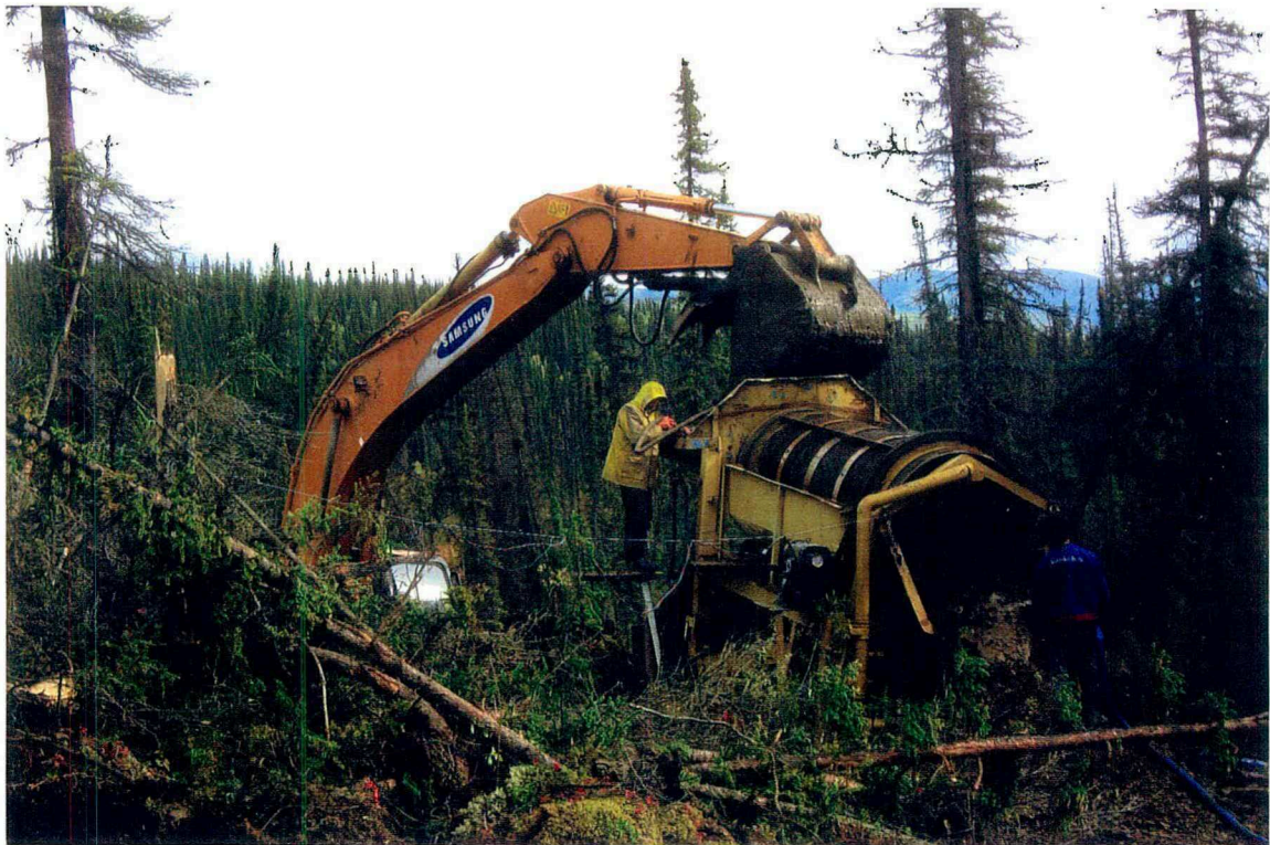
Bulk sampling Black Muck containing sand/gravel seams - Placer claim Mule 2
