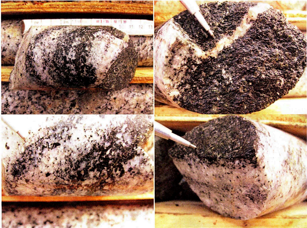
Figure 3: Strongly magnetic foliated mafic rich zones commonly associated with mineralization. These zones were intersected in KSTL-10-02 and KSTL-10-04.
