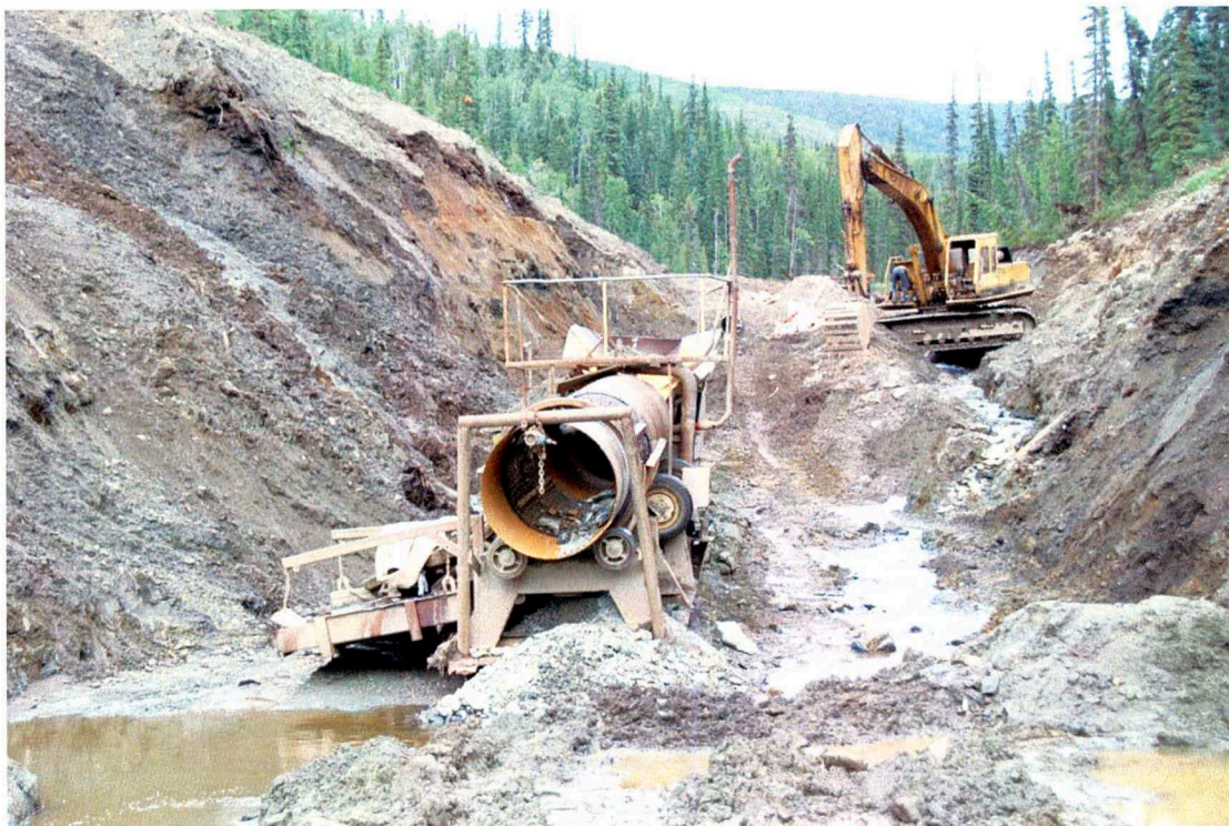
Plate 5 - Trommel wash plant and Caterpillar 235 excavator
