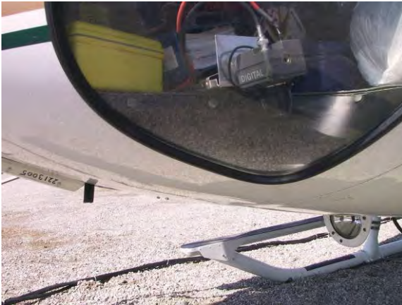
Figure 7. Digital video camera typical mounting location.
