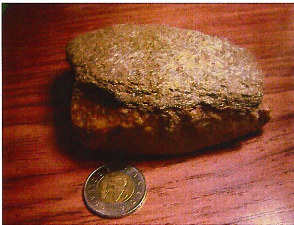
Figure 3. Rusty quartz attached to schist found in hole 7 gravel layer.
