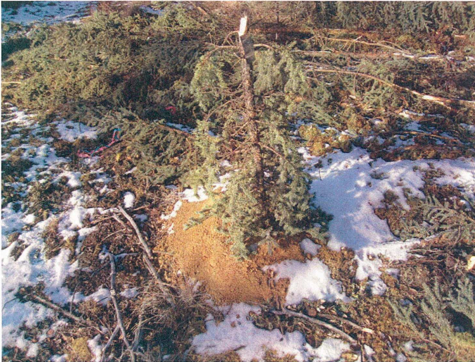
Figure 7. Photograph of completed auger drill soil sample site. The photo shows the rusty, oxidized soil characteristic of anomalous gold values.
