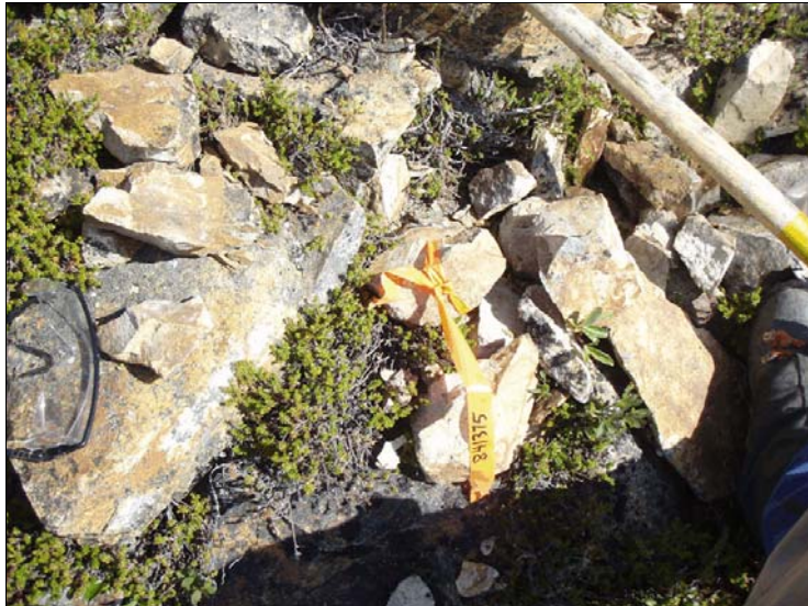
Figure 30. Sn bearing quartz vein (Sample I841375 / 1.550% Sn).
