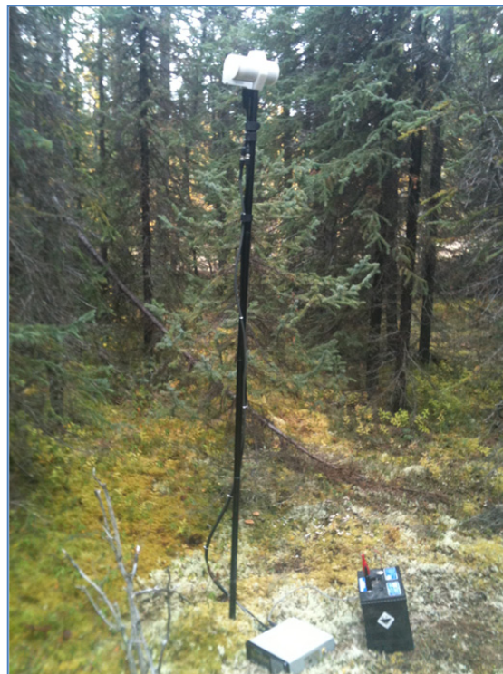
Figure 2 - Mag Base Station setup
