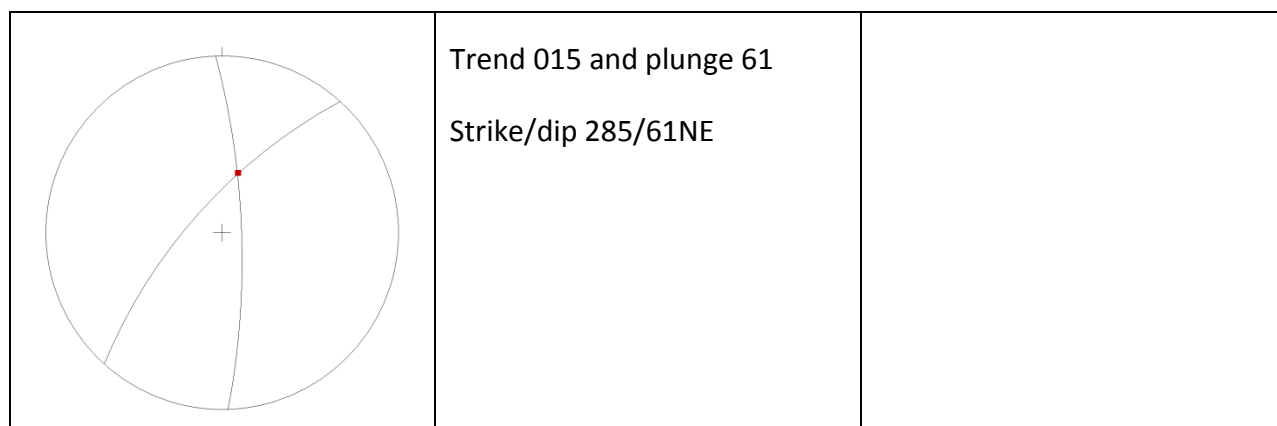
Figure 27: Intersection of the main mineralized vein set with the controlling fault set
