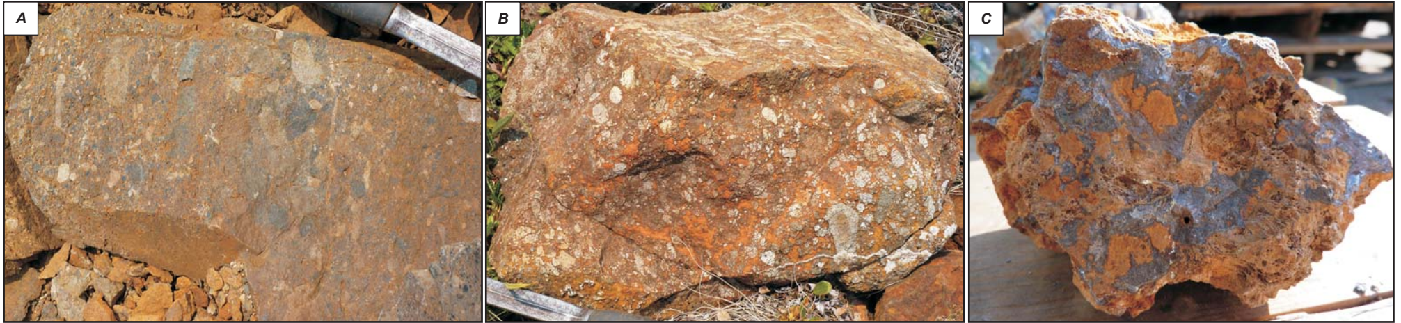
Progressive Fe carbonate alteration of Conglomerate unit and galena replacement of matrix with mineralized zone →
