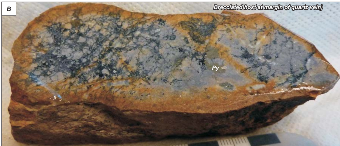
Figure 5: (a) Surface trace of quartz vein located at lithological contact (shale and mafic volcanic?). (b) Brecciation of host (mafic volcanic protolith?) adjacent to quartz vein boundary. (c) and (d) Late stage galena crosscutting early scorodite+ malachite and Scorodite +Qtz (lower elevations).
