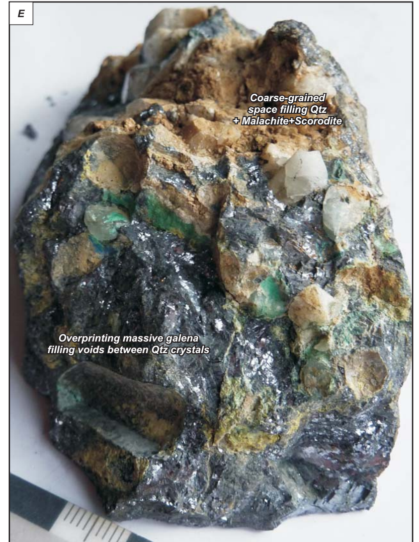
Figure 6: (d) Margin of quartz vein crosscutting mafic volcanic sequence. Coarse grained space filling quartz crystal growth. (e) Coarse grained space filling Qtz+Malachite+Scorodite overprinted by massive Galena.
