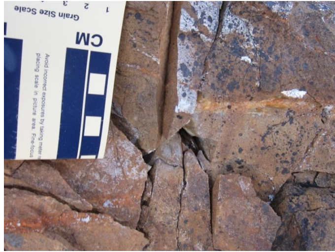
Photo 11: Showing D2 vein (024°/47°NW) cut by D4 faults oriented at 126°/34°SW and 113°/36°SW (not shown). Movement is normal. Offset is between 4 cm and 6 cm.
