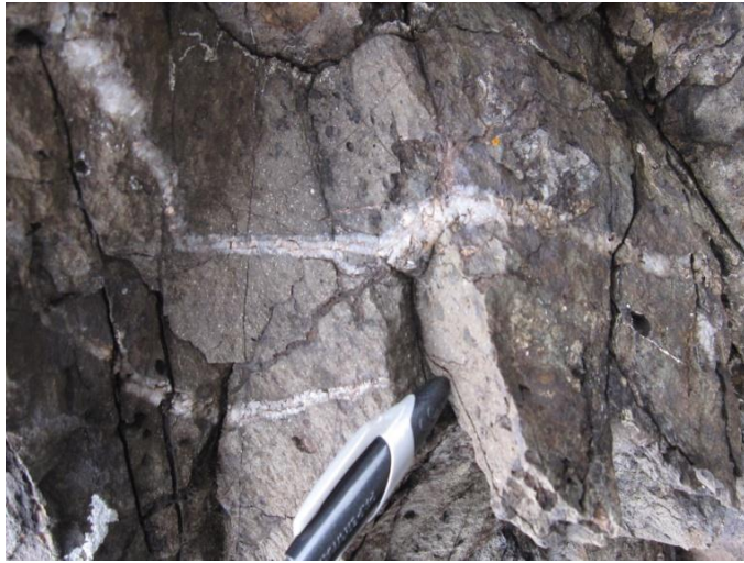
Photo 5: Showing D2 veining in the andesite. Vein oriented at 175°/81°NW.
