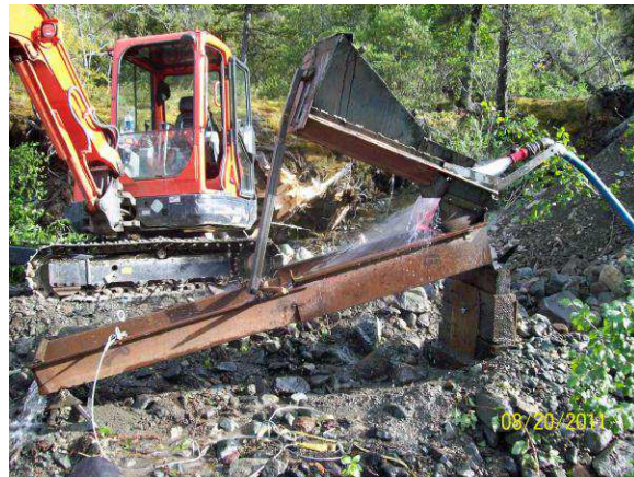
Plate 5: Sluice box used to concentrate gravels
