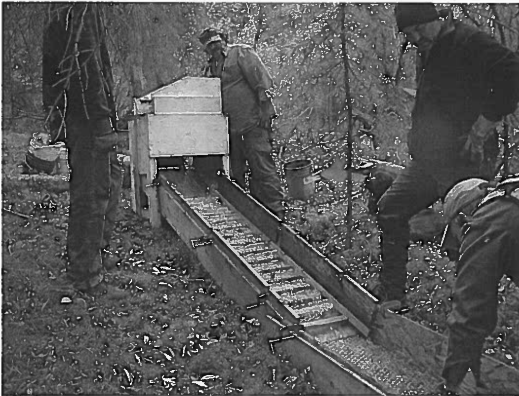
Derek Torgerson and Jeff Bond (Yukon Geology) check out the performance of the sluice box during a test run in 2011.
