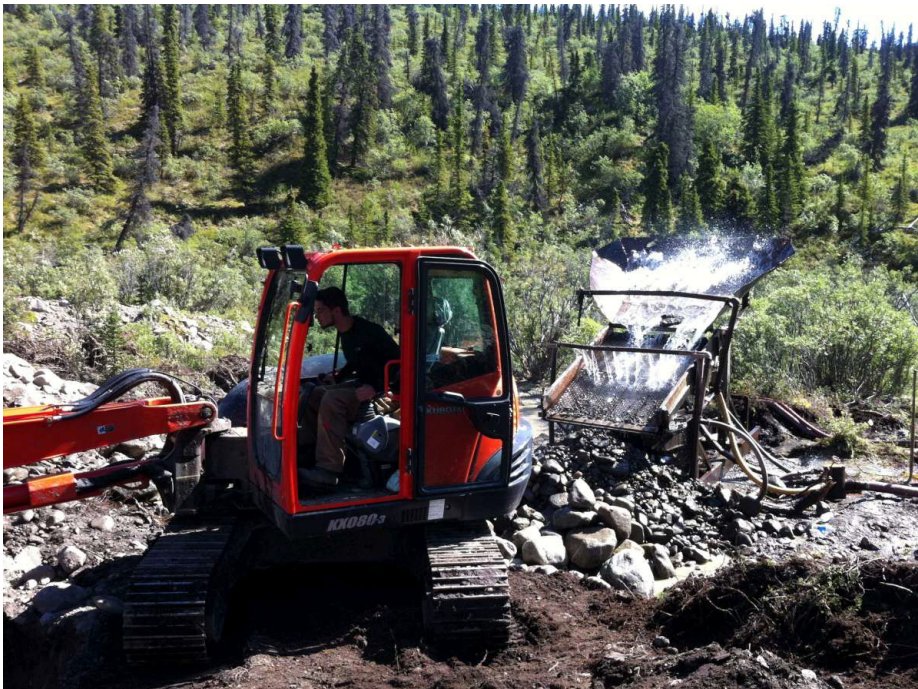
Sluicing at Test Pit 1
