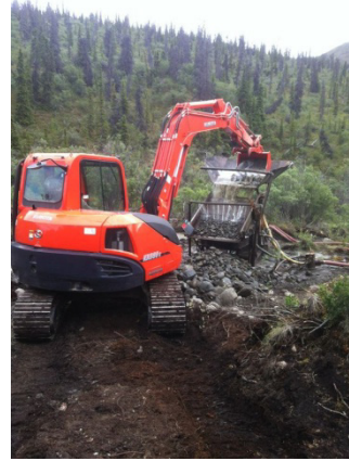
Running gravel through the shaker sluice at pit 1
