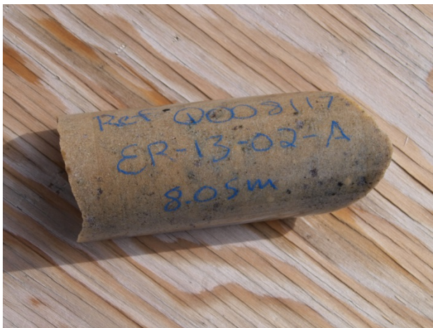
Fig. 3: Alteration zone showing absence of biotite . From reference sample ER-13-02-A
