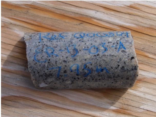
Fig. 5: Grey alteration. Reference sample ER-13-03-A
